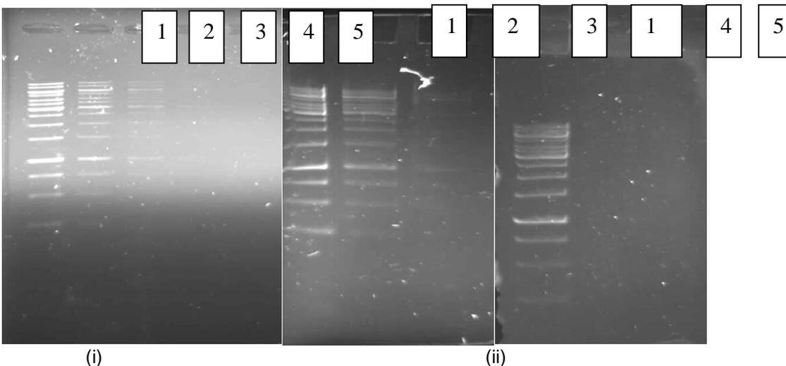
Figure 3: Sensitivity and resolving ability test for (i) Conventional electrophoresis system (ii) Prototype seven (Circuit board) (Lane 1=0.1 µg/µl, Lane 2=0.033 µg/µl, Lane 3=0.011 µg/µl, Lane 4= $3.67 \times 10^{-3}$  µg/µl, Lane 5= $1.22 \times 10^{-3}$  µg/µl)
