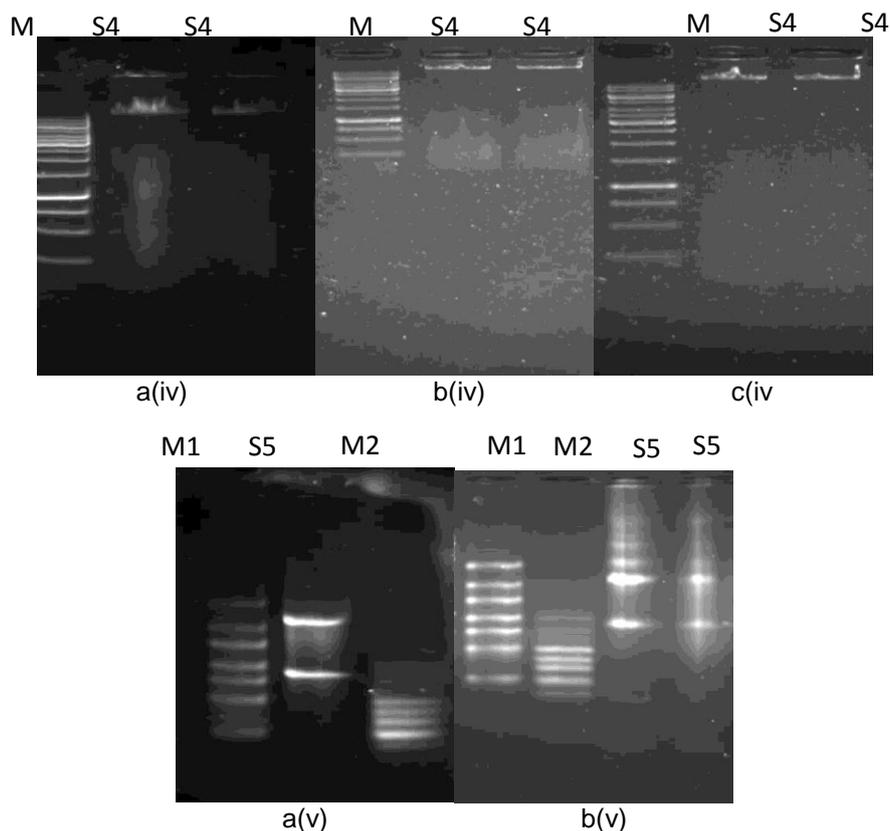
Figure 4: The migration of 5µl of sample DNA bands of different sizes (i) 1700 bp (pcDNA DSN-1)(Lane S1), (ii) 500 bp (Toxoplasma gondii) (Lane S2), (iii) 150 bp (PPARγ) (Lane S3), (iv) 17414 bp (Genomic) DNA of Toxoplasma gondii (Lane S4) and (v) RNA of TW01 NPC cell line (Lane S5) in (a) Prototype seven (circuit board coupled) and (b) conventional unit for 1 hour and in (c) conventional unit for 2 hour (M= DNA marker, M1= High range RNA marker, M2= Low range RNA marker)
