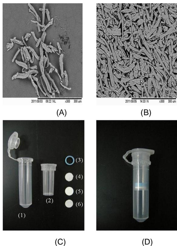
Figure 1: Assembly of spin column. (A) SEM image for cellulose powder before compaction, under 300 x magnification. (B) SEM image for an intact filter disc after compaction, under 300 x magnification. (C) Spin column before assembly: (1) collection tube; (2) minicolumn; (3) O-ring; (4) membrane holder; (5) disc-shaped filter; (6) membrane holder. (D) A complete spin column.
