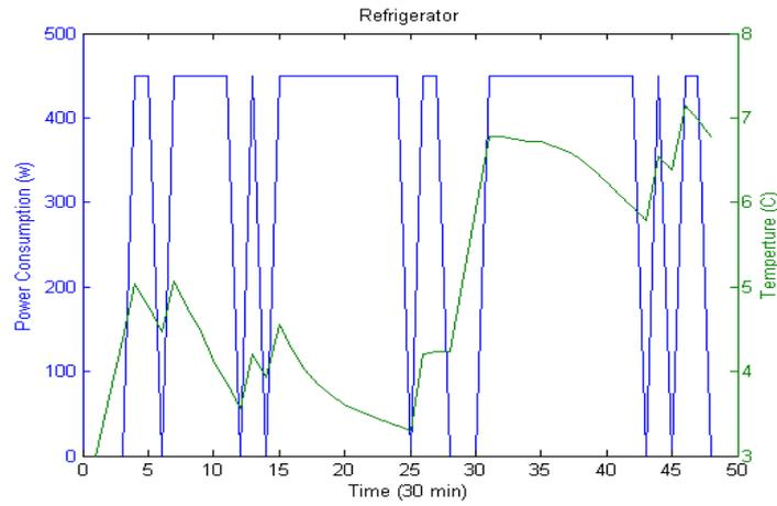
Figure 4: temp and power of refrigerator
