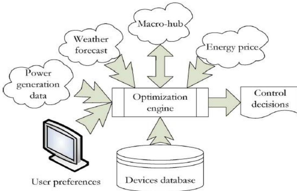
Figure 2: a view of central hub controller
