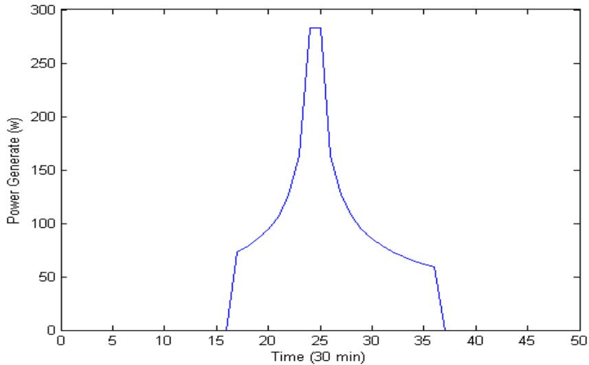
Figure 10: generation power of solar panel
