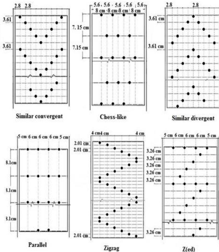
Figure 1. Plan of Arrangement Obstacles
