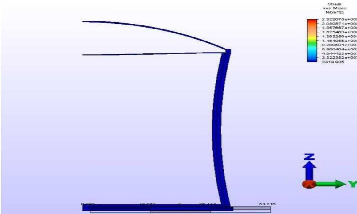
Figur 2: Investigating LNG vessel stress by concave tank wall
