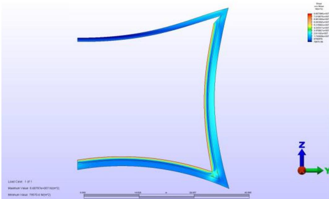
Figure 4: Investigating LNG vessel stress with concave vessel shell
