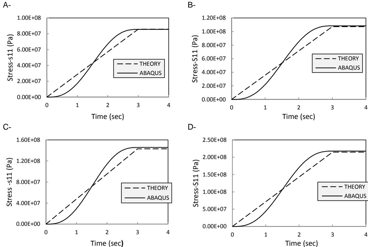
Figure- 6 Comparison of the increasing trend of circular stress in the middle elements of the width of the sheets in the vessel a) mm t=20 b) t = 16) c) t=12 mm d) t= 8mm
