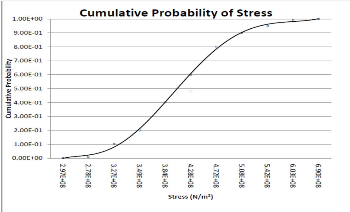
Figur 1: stress investigation in different uncertainties of LNG vessel
