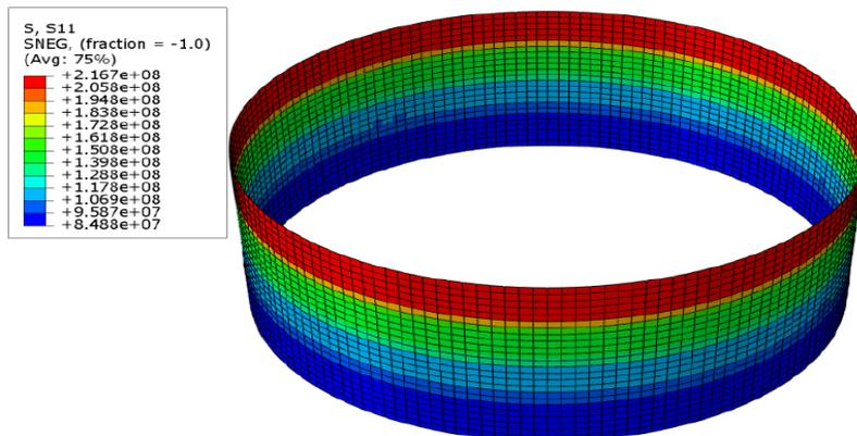
In addition, elements are considered in the middle of each row of the vessel wall sheets and compare the increasing trend of circular stress with theoretical value.
