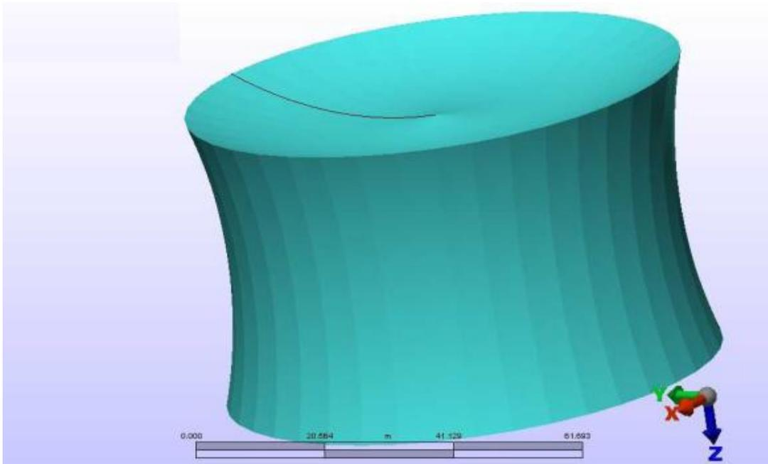
Figur 3. LNG vessel with concave vessel wall
